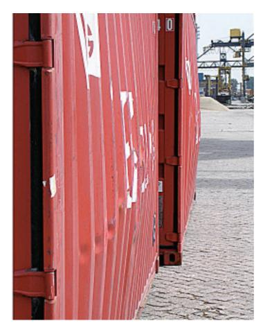
The International Standard Organisation (ISO) / Institute of International Container Lessors (IICL) deformation limit for sidewall panels is a maximum of 10mm beyond the plane of the side surfaces of the corner casting fittings.
