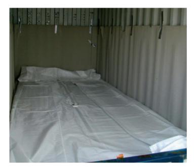
To prevent a loaded flexitank bulging outwards when the right-hand door is open, a false bulkhead is placed in the doorway.
