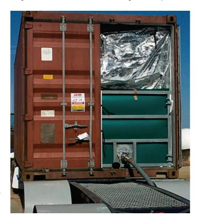
To ensure that a flexitank does not bulge through the gaps in a steel framework bulkhead a sufficiently rigid sheet should be placed on the inside of the bulkhead. This prevents the flexitank chafing against the steelwork. The photograph below shows horizontal steel bars used with cardboard sheeting placed between the flexitank and the steel bars.
