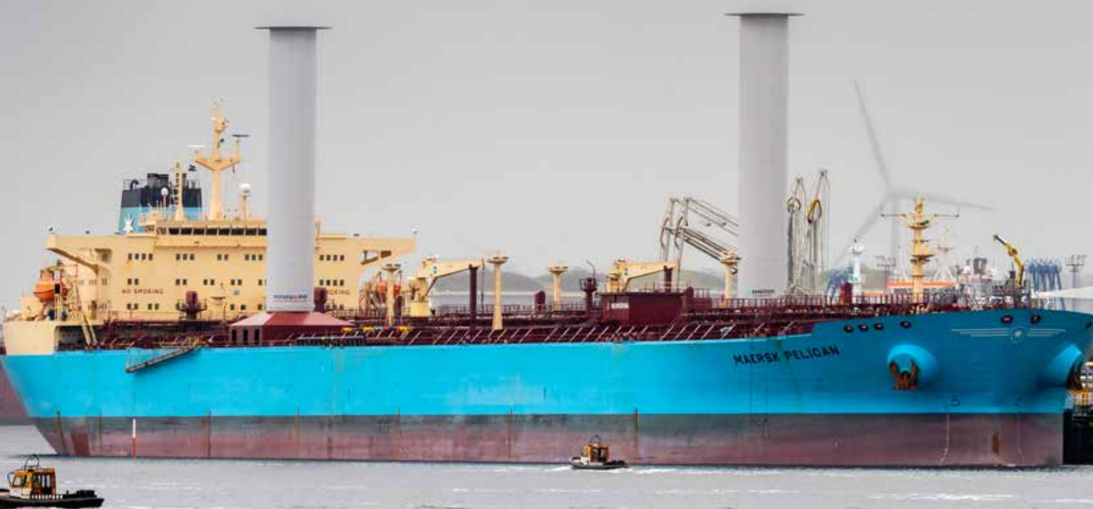
Pictured: the Maersk Pelican equipped with Flettner rotors. Photo credit: Wilsca under the Creative Commons Attribution Share Alike License v4
