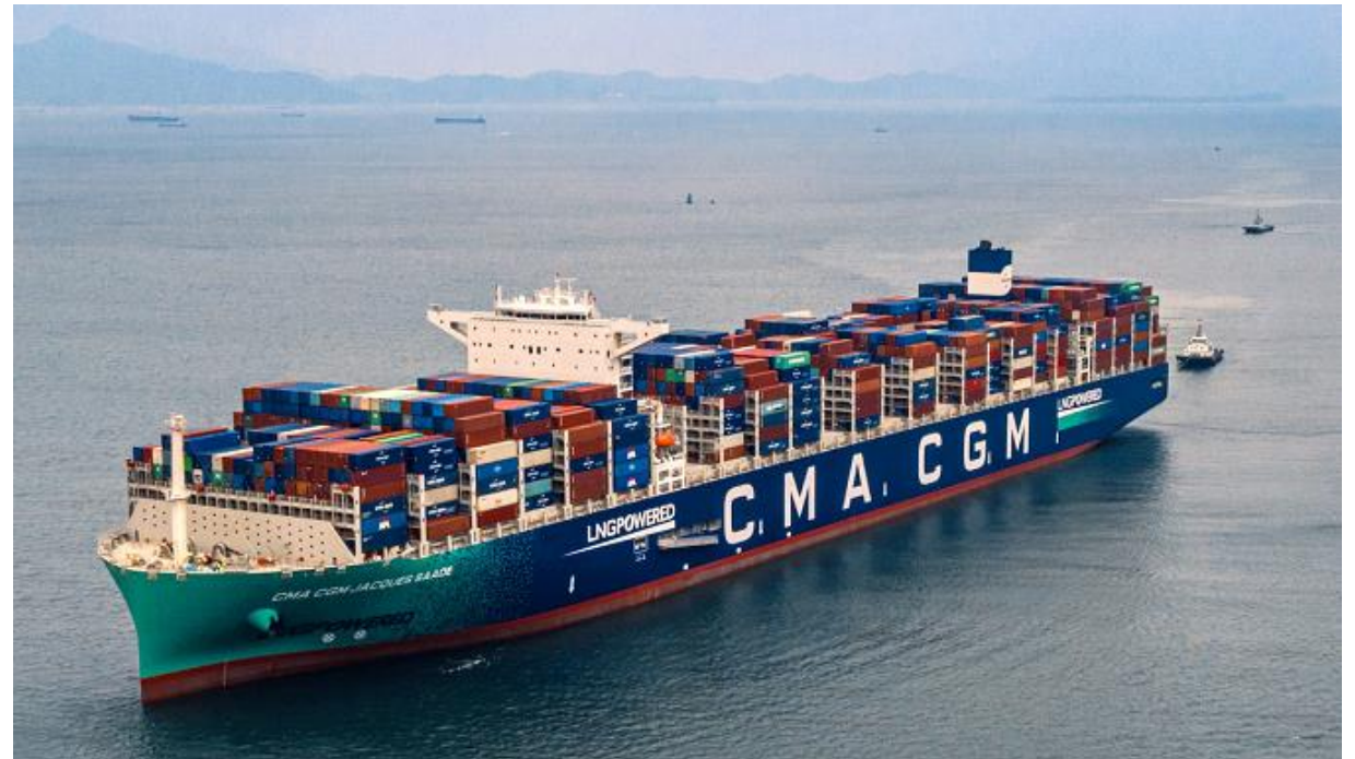
The "Jacques Saade", a 23,000 TEU LNG-powered boxship delivered in 2020. Photo: CMA CGM. Data sources: SEA LNG, Clarkson Research, DNV, IGU
