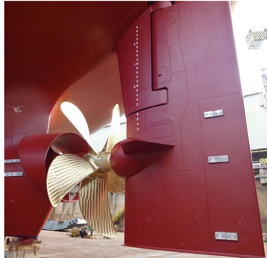
Pictured: a Mewis duct and a rudder bulb installed on a dry bulker. Credit: Oldendorff Carriers.
